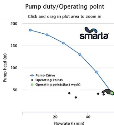
Figure 3 Pump duty points indicate selection criteria for solar pump
