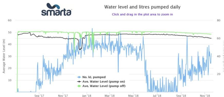
Figure 1 SMARTA logs water volumes pumped and borehole water levels from farm borehole
