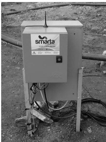
Figure 15 SMARTA Logger and Reader enclosure mounted
