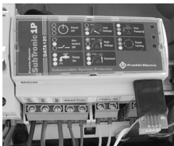
Figure 9 Fit infra-red bracket to SubTronic control box/panel
