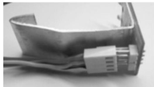
Figure 10 How to connect the infra-red port
